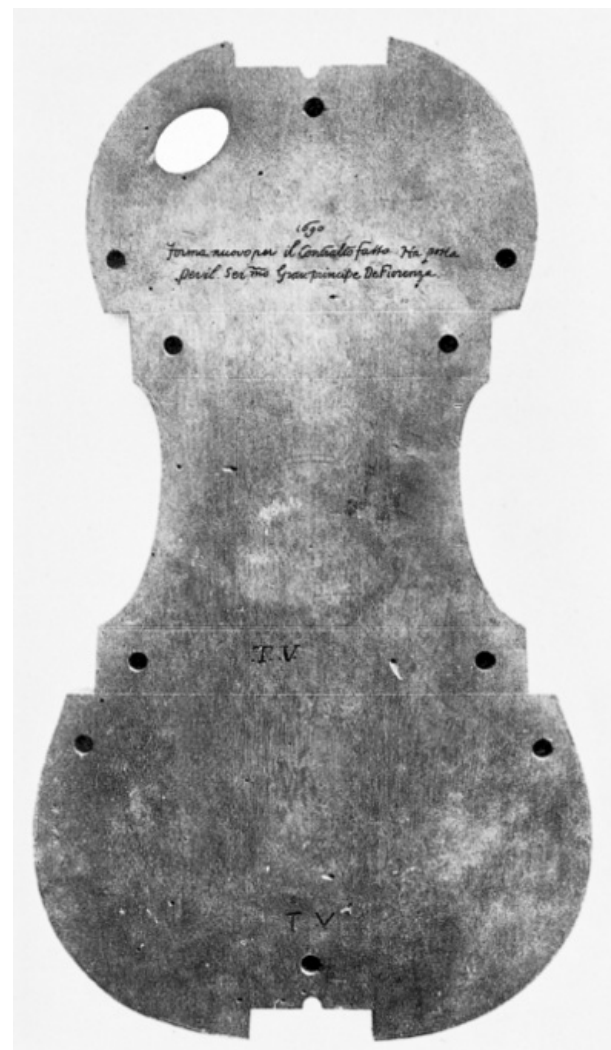
FIGURE 6. One of Stradivari’s internal molds, in this case for a tenor viola.
